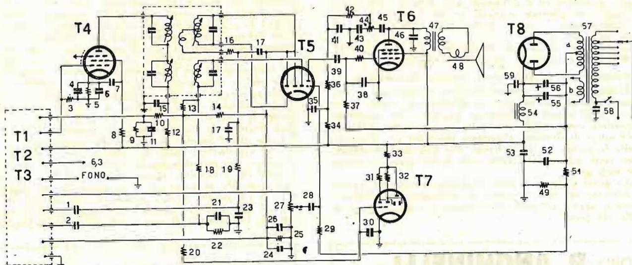
TUBI - T1 - EF80; T2 - ECC81; T3 - ECH81; T4 - EF85; T5 - EABC80; T6 - EL84; T7 - EM34; T8 - EZ40.
